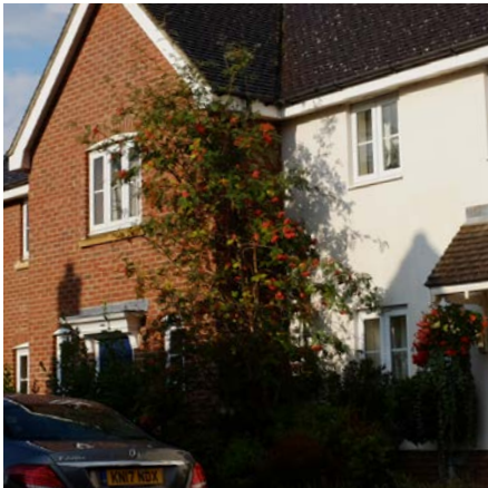
A recent housing development; the community has preference for brick over rendered dwellings as render tends to wear less well in this context.
